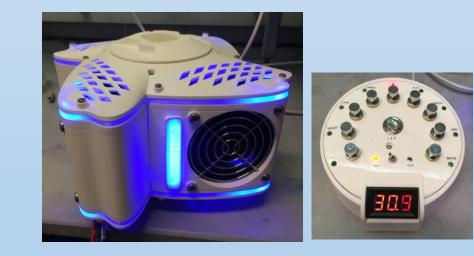
Left:ThePhotoCubeTMProPrototype (indicated as R2 on theflow graph above) in operationduring a Minisci reaction.Right:
